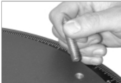
Fig. 47: Remove the pointed bolts from the drive base.
