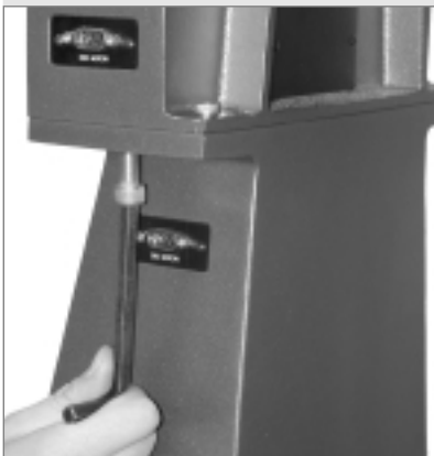
Fig. 53: Tighten the fork arm assembly using the provided hex key.
