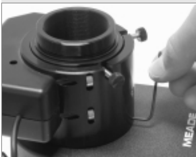
Fig. 60: Tighten the three microfocuser hex screws to a firm feel.
