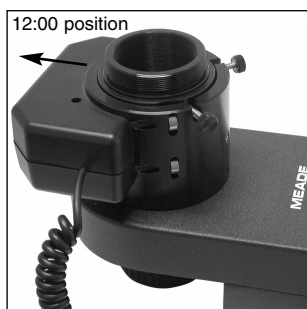
Fig. 8: Place the microfocuser over the adapter ring. Notice the orientation of the microfocuser.
