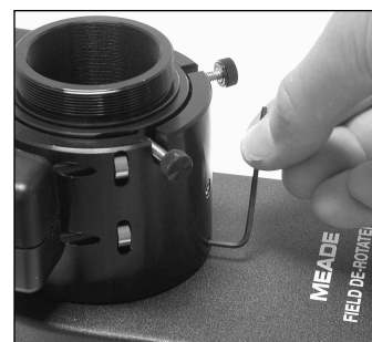
Fig. 9: Tighten the three microfocuser set screws to a firm feel.
